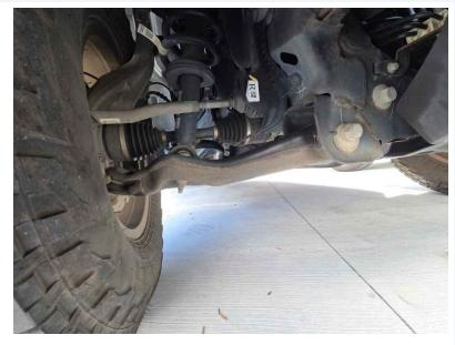
wheel bearing suspected for mild hum, though cannot be confirmed without a lifting test.
